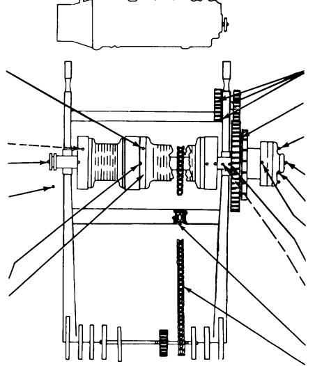
10 CW11 Intermediate Hoist and **Pinion Shaft Gears** 10 GAA Safety Pawl Pin (3 fittings) 10 GAA Planetary Pinions (2 fittings) 100 GAA Drum Shaft Outboard **End Bearing** 10 GAA Planetary Spider 100 GAA Boom Hoist Drum Bear-100 GAA Drum Shaft Bearing 250 GAA Clutch Drum Bearing Plug (Remove plugs and insert fitting to lubricate) GAA Chain Tightener
